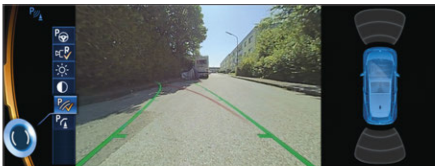
Rear view camera, view in CID with parking assistance lines
